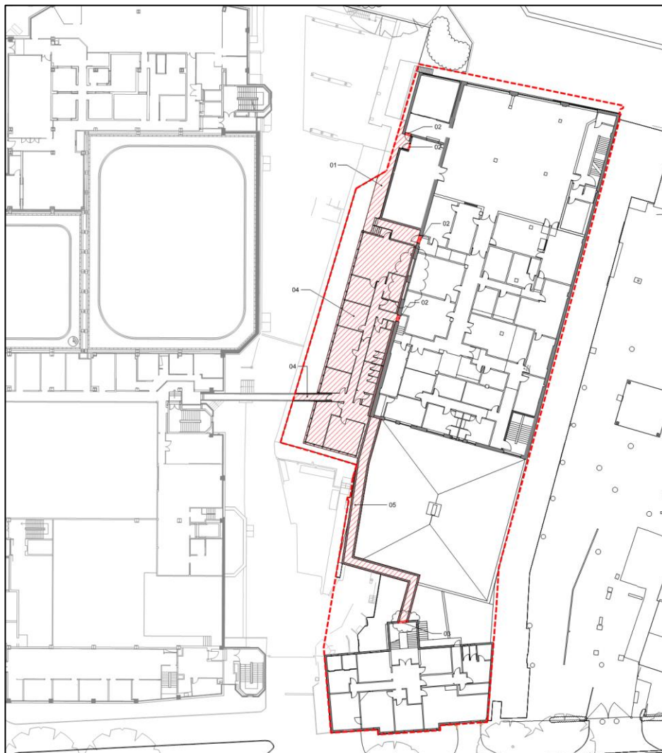
Figure 1: Structures to be demolished
