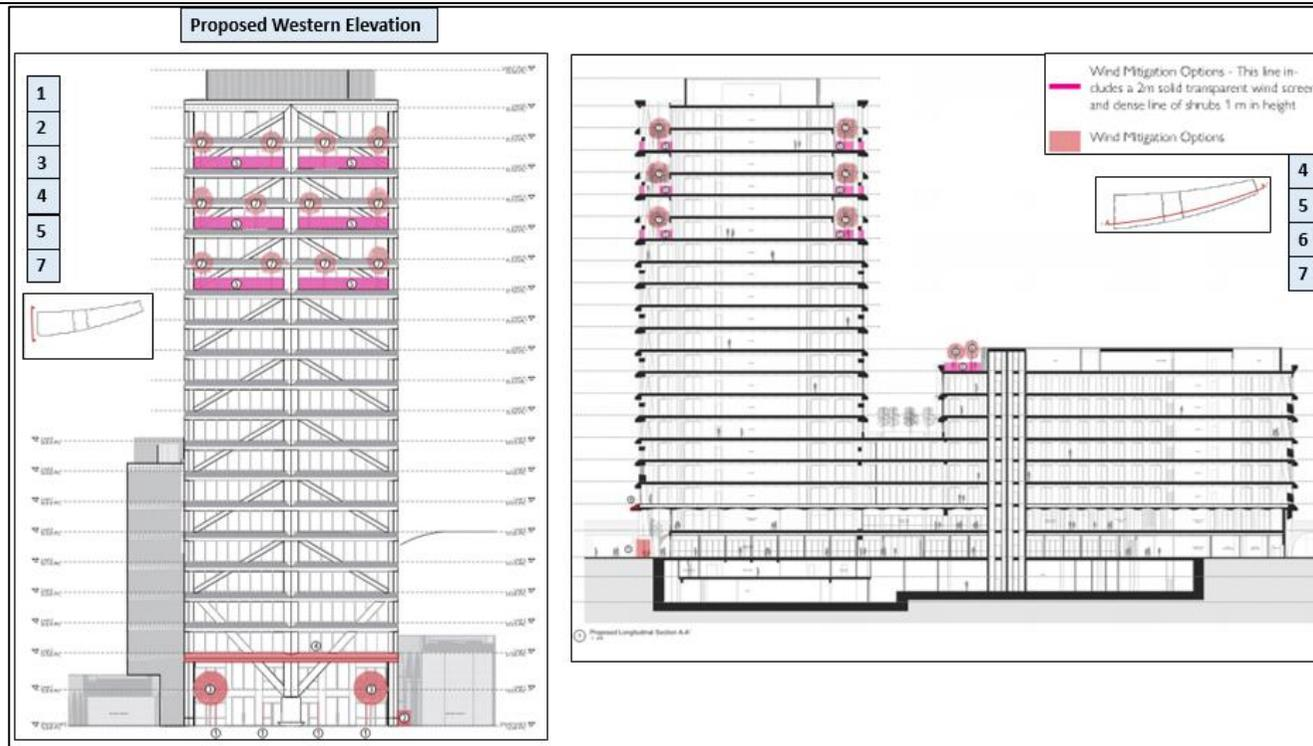
**Figure 8** – Proposed wind mitigation measures (Mitigation Measures 2, 3, 4, 5, 6 and 7) on the western elevation and long section
