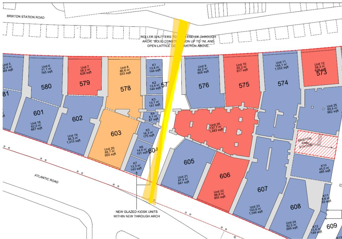
2.22 The new link would be between 3.8m and 4.2m in width at each end. However, owing to the arch structure, there is a narrowing in the middle section down to 1.9m and 2m respectively. This width is sufficient to accommodate a double buggy as well as wheelchairs and mobility scooters.
